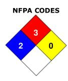
NFPA 30 / 30B Storage Classification: Flammable Liquid IB
